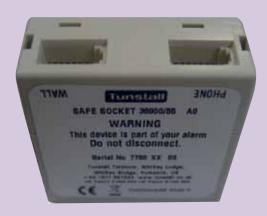
For a Cornwall Lifeline Alarm to provide emergency support it must be able to raise an alarm on the telephone line even when another telephone within the property is being used or has accidentally been left off hook.
