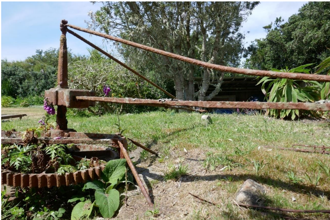
Fig 156 St Agnes: Detail of Lower Town Farm horse-engine, showing the cast iron toothed gear wheels and two arms with their lighter arm stays; and the round-section, wrought iron horse shafts for one of the arms, with fixtures for harnessing. Since it was recorded by CAU (Ratcliffe and Parkes 1990) some iron has corroded away.
