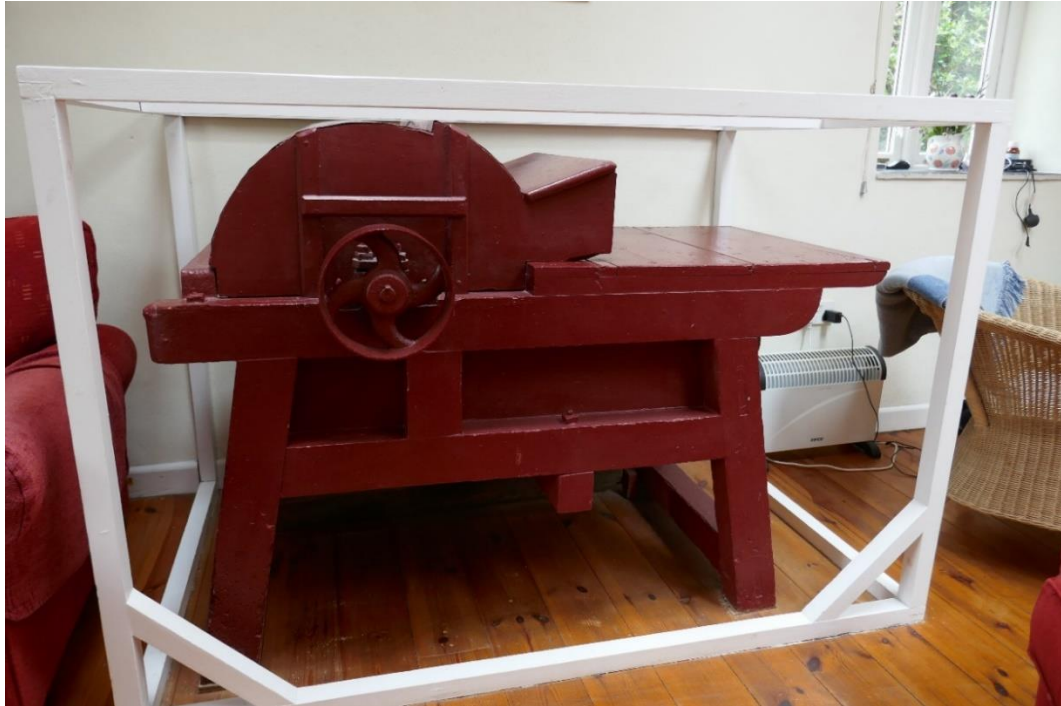
Fig 157 St Agnes: Lower Town Farm barn, thresher on the other side of the wall from the external platform with horse engine which powered this machinery.
