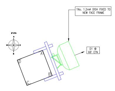
PLAN VIEW OF NEW 1.2mø DISH @ 60.0m MEAN A.G.L (SCALE 1:50)
