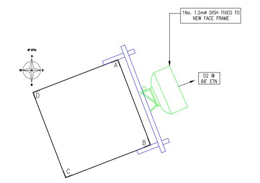
PLAN VIEW OF NEW 1.2mø DISH @ 50.0m MEAN A.G.L (SCALE 1:50)
