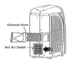
The hot exhaust air can be vented through the wall or out a window. If mounting in the wall, the height of the hole should be 40cm to 130cm.
