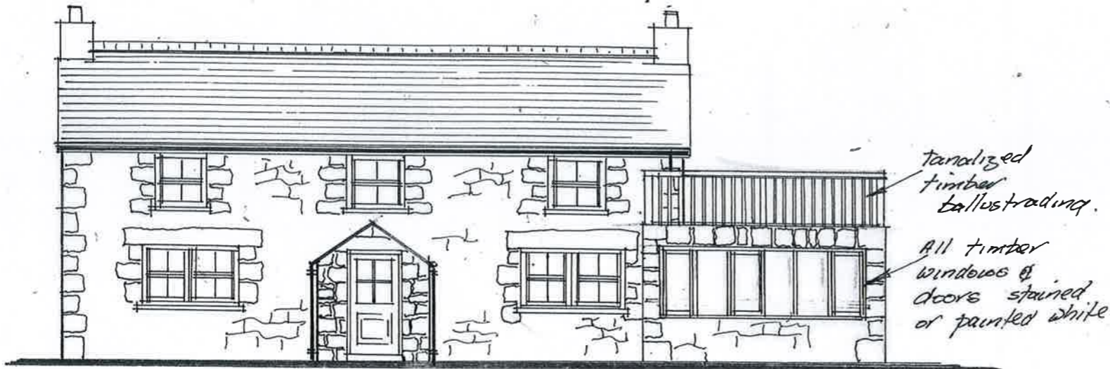
FRONT ELEVATION (WEST)
