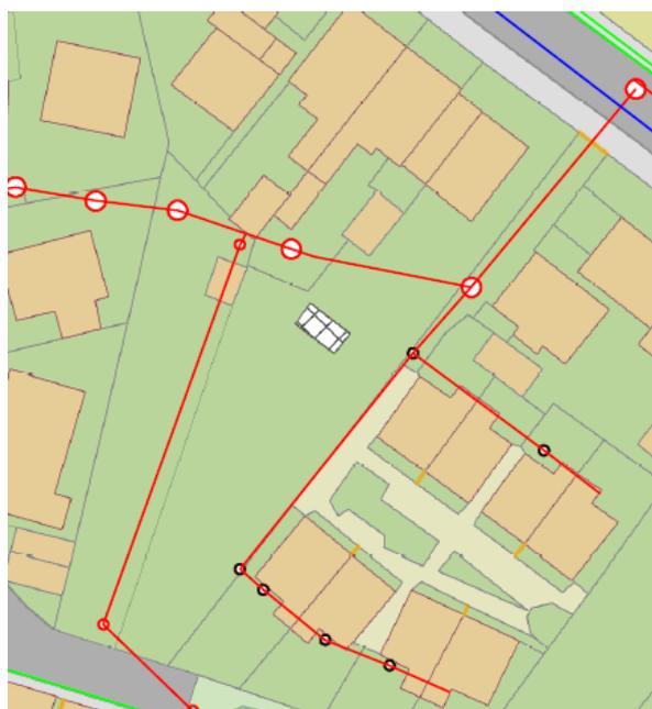
Fig 5. Sewerage network showing takes for proposed property
