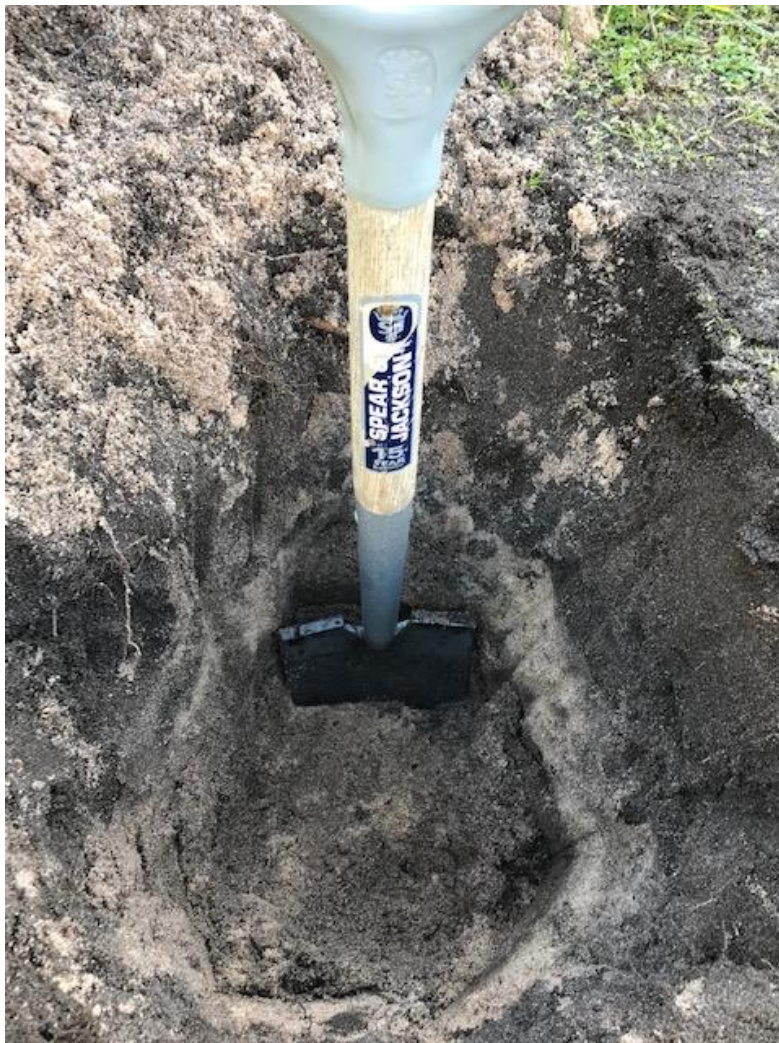
Photograph 01 – showing the soil profile for the first 2ft at the proposed site of the Staff Dwelling on the Vineyard.
