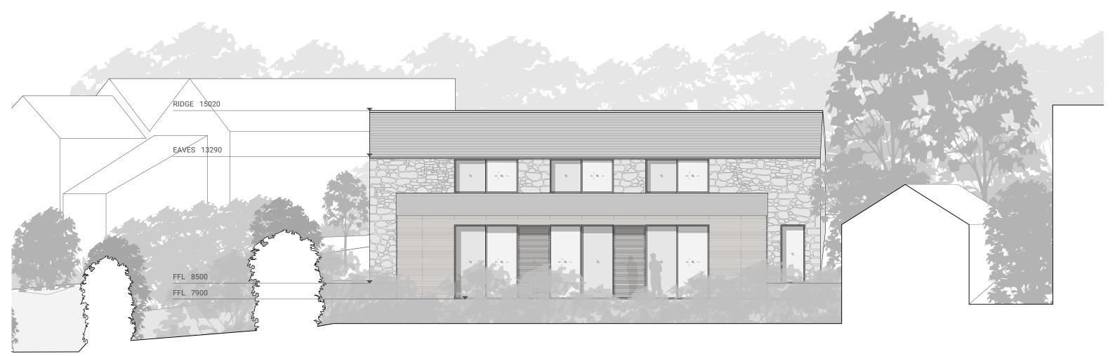
Revision: Date: Item: 14.05.19 Height of house alterations and extension reduced. Stonework and screens added to elevation А
