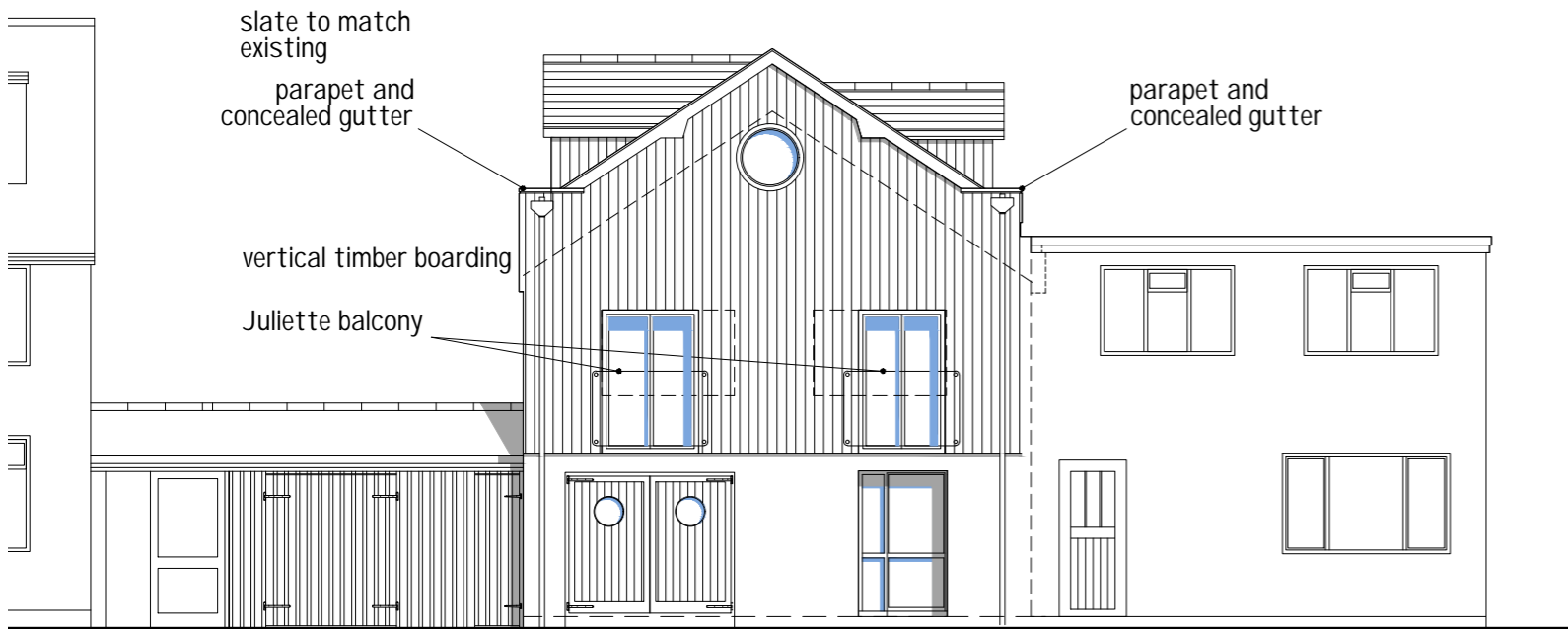
Penlee Boathouse FRONT ( SOUTH ) ELEVATION
