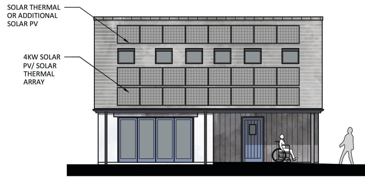
01 SOUTH WEST ELEVATION
