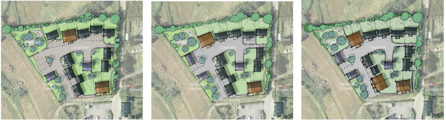
Image 4.4, 4.5 & 4.6 - Three options produced following feedback from the 'Self Build Session' exploring a courtyard approach. All options illustrate 13 plots.
