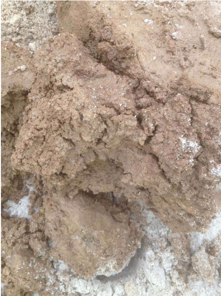
Fig 3 – Trial Pit 1 – Sand / Gravel / Clay composite
