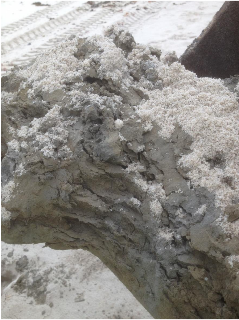
Fig 13 – Pit 3 – Clay in swing shovel
