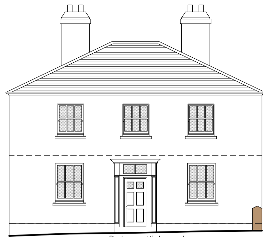
Front Elevation [East Facing] - Proposed
