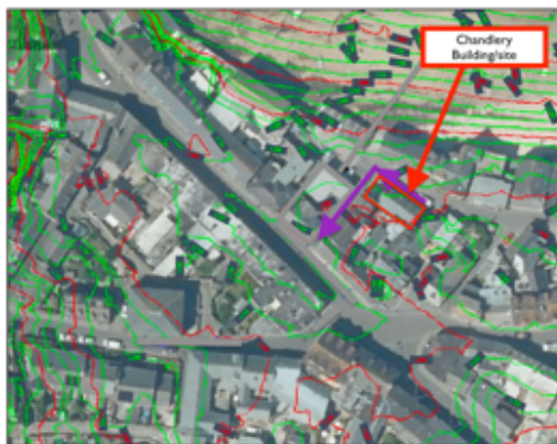
Figure 5 – Contour data from LiDAR including the Preferred Access/Egress route for the Site
