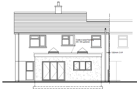
REAR (NORTH) ELEVATION
