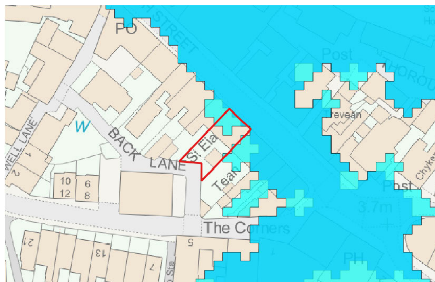
Figure 2: Flood mapping from the EA online data. The site falls within Flood Zone 3
