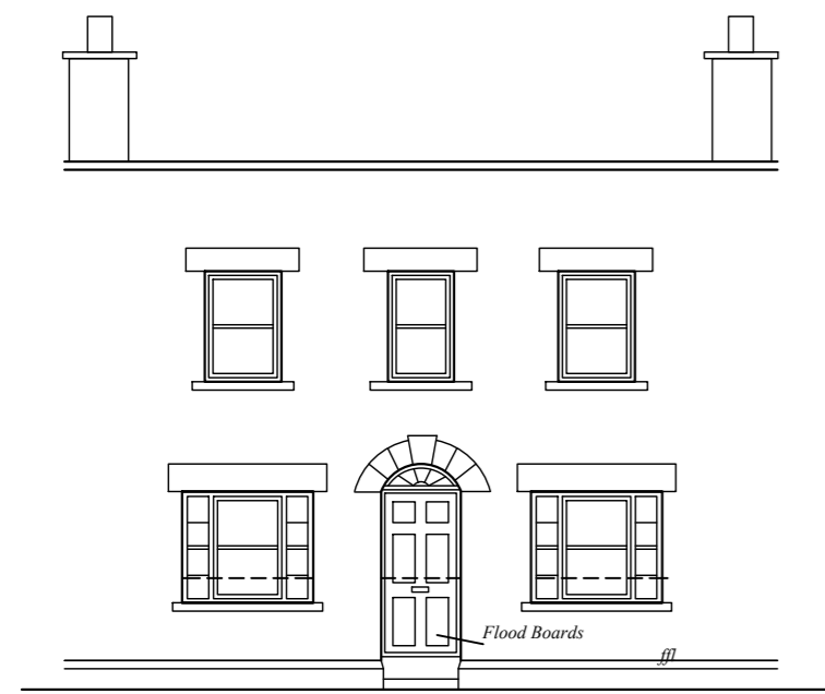
East Elevation (Front)
