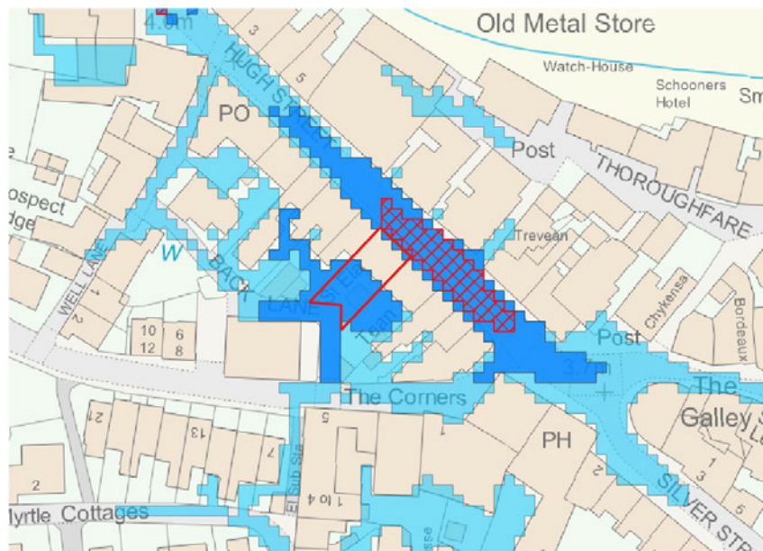
Figure 4: SW flood extent mapping. The front of the site is shown to be at a High risk from SW flooding.
