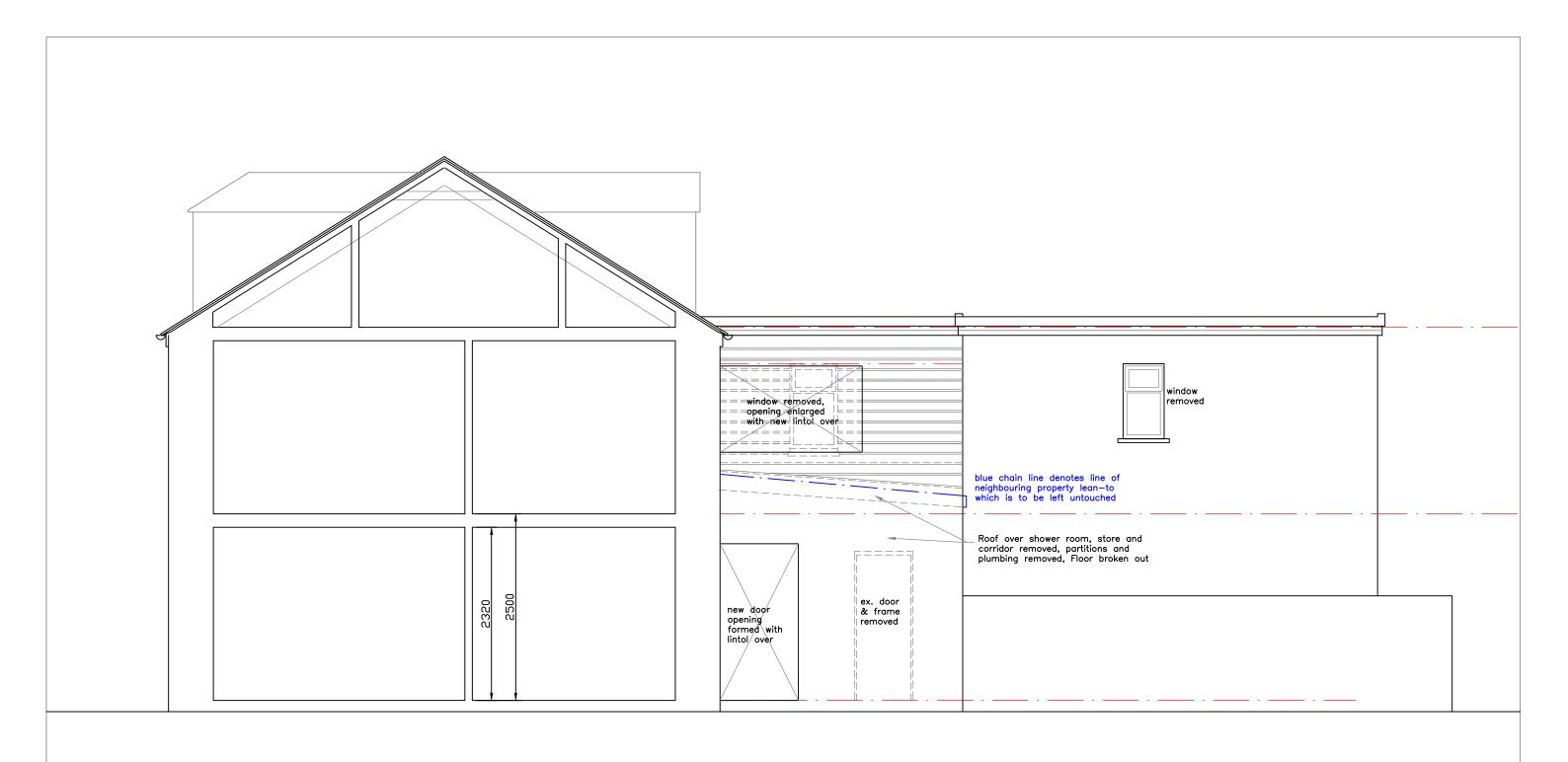
Alterations to Wingletang, St. Mary's for EGV Consulting Ltd West elevation proposed demolitions
