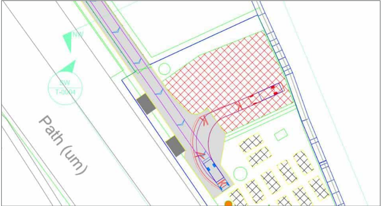
Figure 4.8: Vehicle tracking of 9.5m delivery vehicle using turning head
