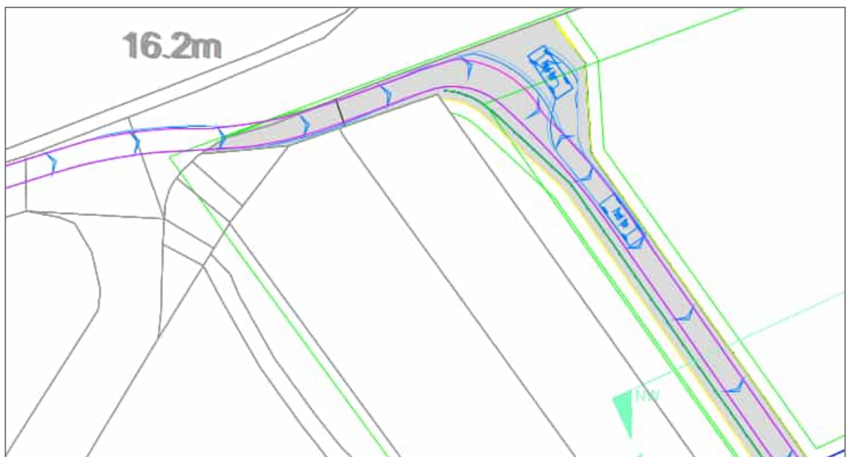
Figure 4.5: Vehicle tracking of 9.5m delivery vehicle entering site passing waiting minibus
