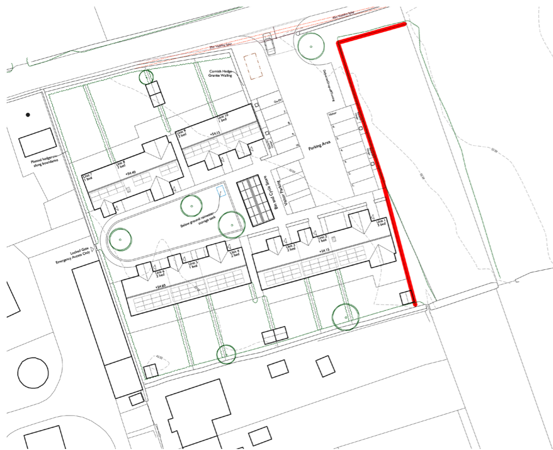
Line of Tree Protection Fencing highlighted in red
