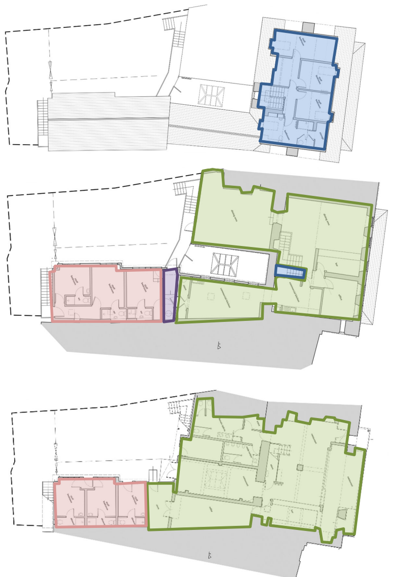
Figures 2-4: 'Existing' floor plans indicating trade areas at ground, first and second floor levels.
