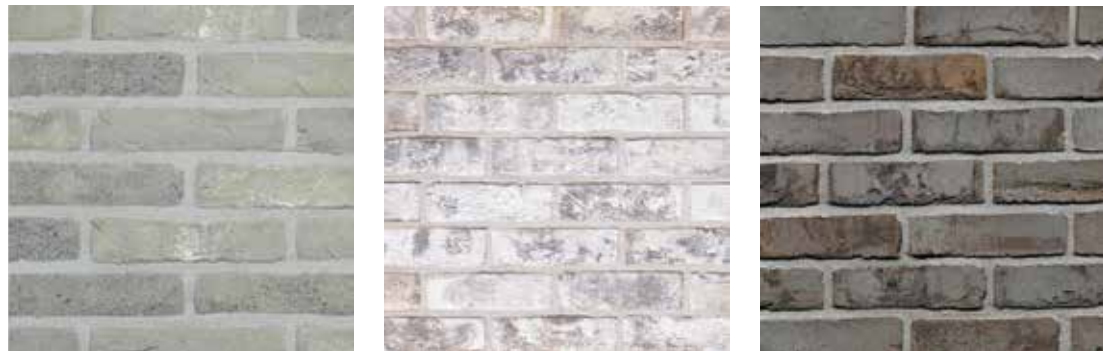
possible options for a grey-multi brick with colour matched mortar used as low level plinth
