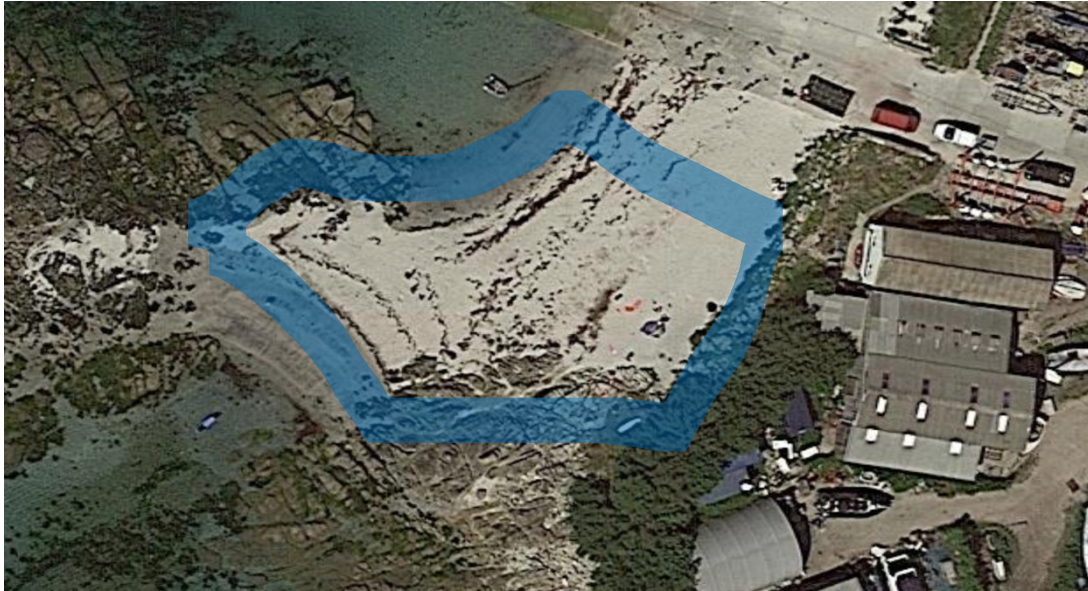
Figure 4. Redistribution of materials on sea front. Sand bar highlighted in blue.
