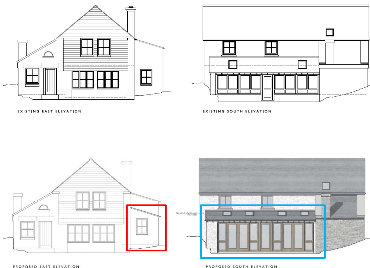
Figure 2: Excerpts from the existing plans (top) and proposed plans (bottom) showing the areas to be impacted by the proposed development. Red outline shows the proposed single-storey extension on the north elevation. Blue outline shows the proposed replacement sunroom on the south elevation.
