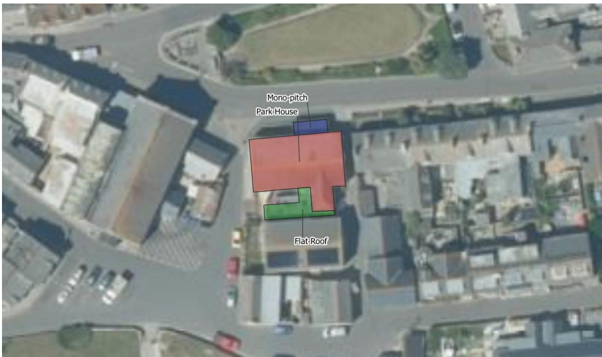
Map 02 – Showing the main Park House structure indicated by the red wash with the monopitch roof indicated to the front in the blue wash; and the flat-roof component to the rear indicated by the green wash.
