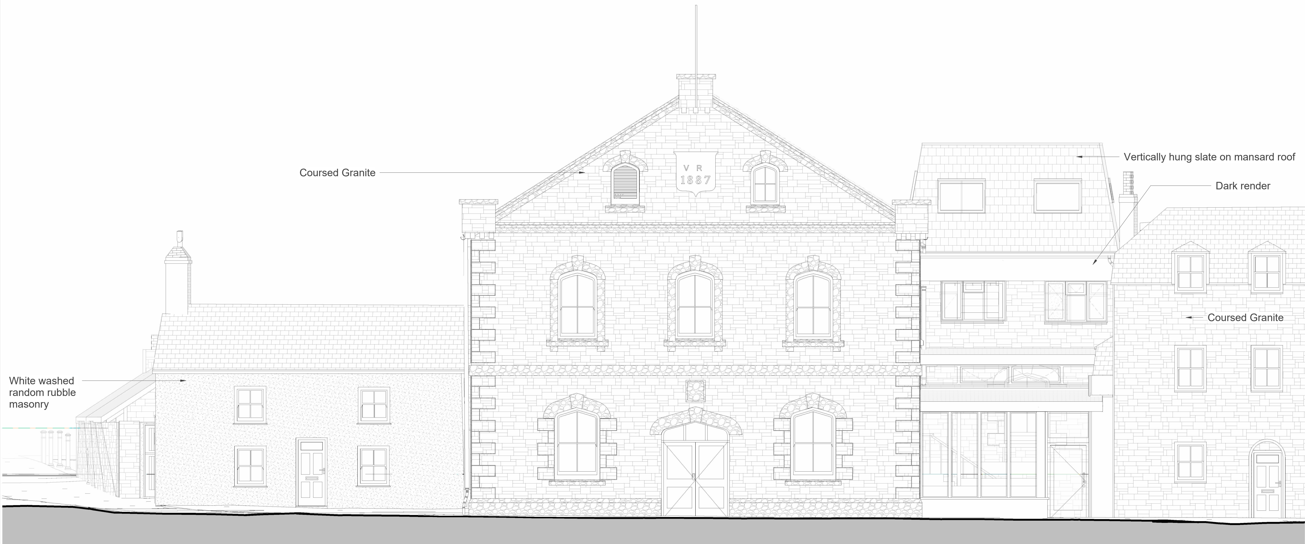
1 Planning North East Elevation - Existing 1 : 50
